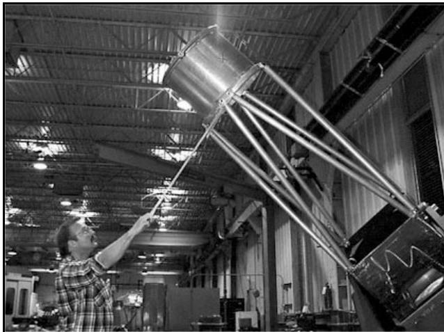
**Brad pulls on the strap, and "tames" the telescope. Until the optics are installed, the telescope assembly is out of balance and needs to be carefully maneuvered.**
