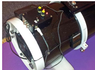
Cooling fan, a dew controller, a Li-ion battery and mirror/ambient thermometer mounted on a 10" Newtonian Telescope.
